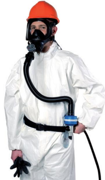
The **TR 82** full face mask with panoramic visor is connected to the overflow valve that releases the excess air to the external environment. The mask is fed by the **TUR 801** corrugated hose which draws breathable air in the respiration zone and which is positioned between the overflow valve and the filter silencer connected to the flow regulator.
